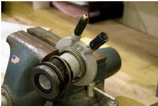
**1.2** With the CSC body held in the position described in step (a), hold the inlet tube and the bleed tube straight up (vertical).
